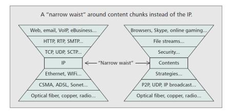
Figure 2. The new "narrow waist" of NDN (right) compared to the current Internet (left) [7]
